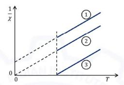
(Curie temperature of ferromagnetic material = $T_{\rm C}$ Néel temperature of antiferromagnetic material= $T_{\rm N}$ )
