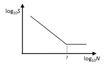
The life of a cylindrical shaft made of this material subjected to an alternating stress of 200 MPa will then be \_\_\_\_\_ cycles (round off to the nearest integer).
