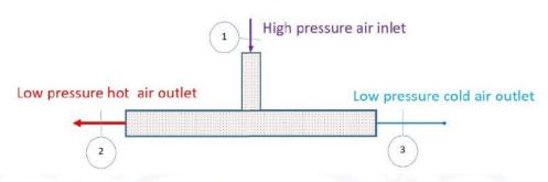
Assume constant specific heat of air is 1005 J/kg.K and gas constant is 287 J/kg.K. There is no work transfer across the boundary of this device. The rate of entropy generation is \_\_\_\_\_kW/K (round off to one decimal place).
