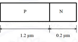
The magnitude of reverse bias voltage that would completely deplete one of the two regions (P or N) prior to the other (*rounded off to one decimal place*) is V.
