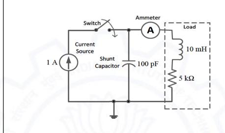
Initially, when the switch is open, the capacitor is discharged and the ammeter reads zero ampere. After the switch is closed, the ammeter reading keeps fluctuating for some time till it settles to a final steady value. The maximum ammeter reading that one will observe after the switch is closed (rounded off to two decimal places) is А.
