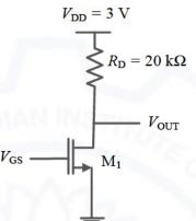
The channel length modulation coefficient is ignored. If the gate-to-source voltage  $V_{GS}$  is 1 V to keep the transistor at the edge of saturation, then the threshold voltage of the transistor (*rounded off to one decimal place*) is \_\_\_\_\_\_ V.
