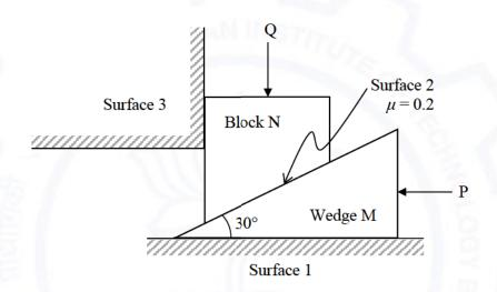
The limiting force P, in terms of Q, required for impending motion of block N to just move it in the upward direction is given as  $P = \alpha Q$ . The value of the coefficient ' $\alpha$ ' (round off to one decimal place) is
