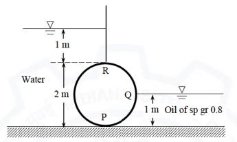
The absolute ratio of the net magnitude of vertical forces to the net magnitude of horizontal forces (round off to two decimal places) is \_\_\_\_\_\_
