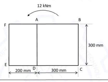
Q.51 Two cantilever beams AB and DC are in contact with each other at their free ends through a roller as shown in the figure. Both beams have a square cross section of 50 mm x 50 mm, and the elastic modulus E = 70 GPa. If beam AB is subjected to a uniformly distributed load of 20 kN/m, then the compressive force experienced by the roller is \_\_\_\_\_ kN (round off to one decimal place).
