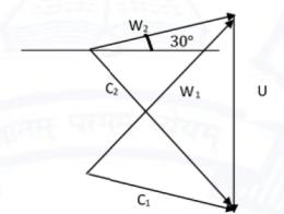
The blade speed (U) at the mean radius of the rotor is \_\_\_\_\_ m/s (round off to two decimal places).
