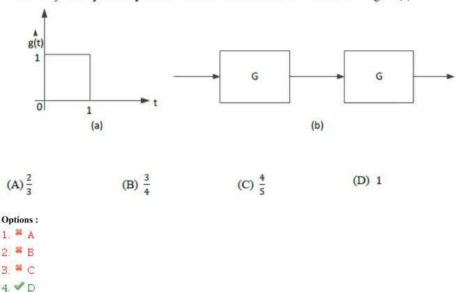
The impulse response g(t) of a system, G, is as shown in Figure (a). What is the maximum value attained by the impulse response of two cascaded blocks of G as shown in Figure (b)?
