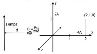
Assuming right handed coordinate system, magnetic field intensity,  $\vec{H}$  at coordinate (2,1,0) will be
