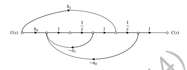
Assuming,  $h_1 = b_1$  and  $h_0 = b_0 - b_1 a_1$ , the input-output transfer function, G(s) =of the system is given by
