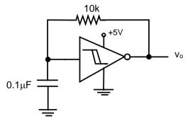
If the lower and upper trigger level voltages are 0.9 V and 1.7 V, the period (in ms), for which output is LOW, is \_\_\_\_\_.
