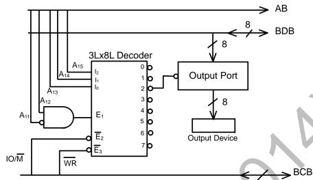
The interfacing circuit makes use of 3 Line to 8 Line decoder having 3 enable lines  $E_1, \overline{E}_2, \overline{E}_3$ . The address of the device is
