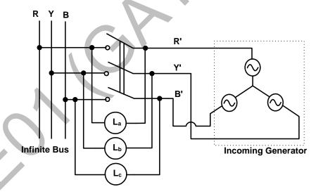
It was found that the lamps are becoming dark in the sequence  $L_a$ - $L_b$ - $L_c$ . It means that the phase sequence of incoming generator is
