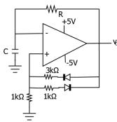
The time duration for +ve part of the cycle is  $\Delta t_1$  and for -ve part is  $\Delta t_2$ . The value of  $e^{\frac{\Delta t_1 - \Delta t_2}{RC}}$  will be \_\_\_\_\_\_.
