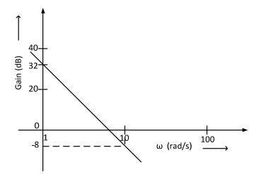
The gain  $(20 \log |G(s)|)$  is 32 dB and -8 dB at 1 rad/s and 10 rad/s respectively. The phase is negative for all  $\omega$ . Then G(s) is
