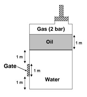
Q.17 The pressure (in bar) exerted on the bottom wall inside the vessel is approximately
